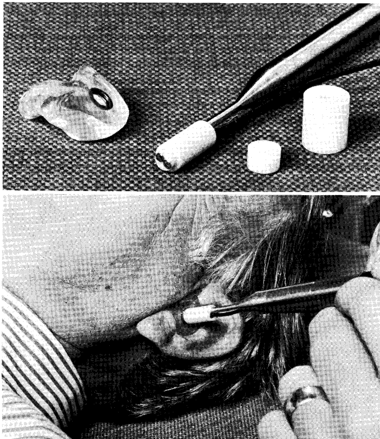
Fig.7. The two 3 mm microphones placed in a holder formed as the hub of a hearing aid earphone for measuring the impedance presented to the earphone together with two reference volumes. Below: impedance measurements on an ear mould placed in human ear
