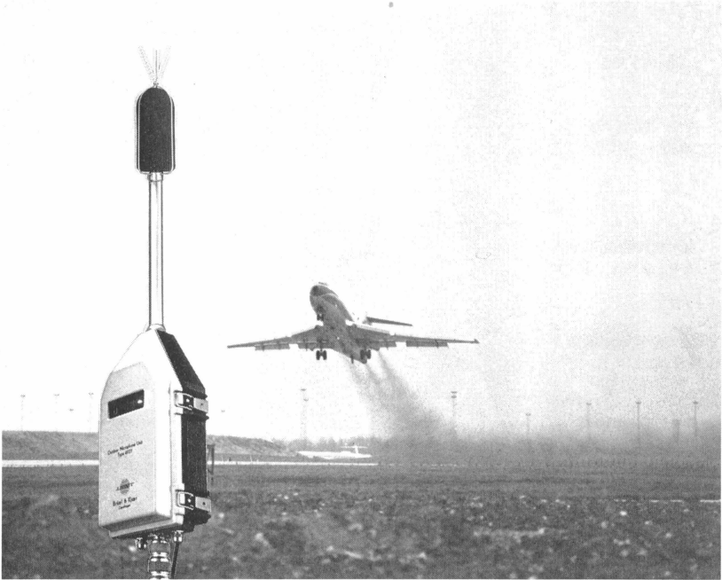
Fig.15. Outdoor monitoring of aircraft noise
