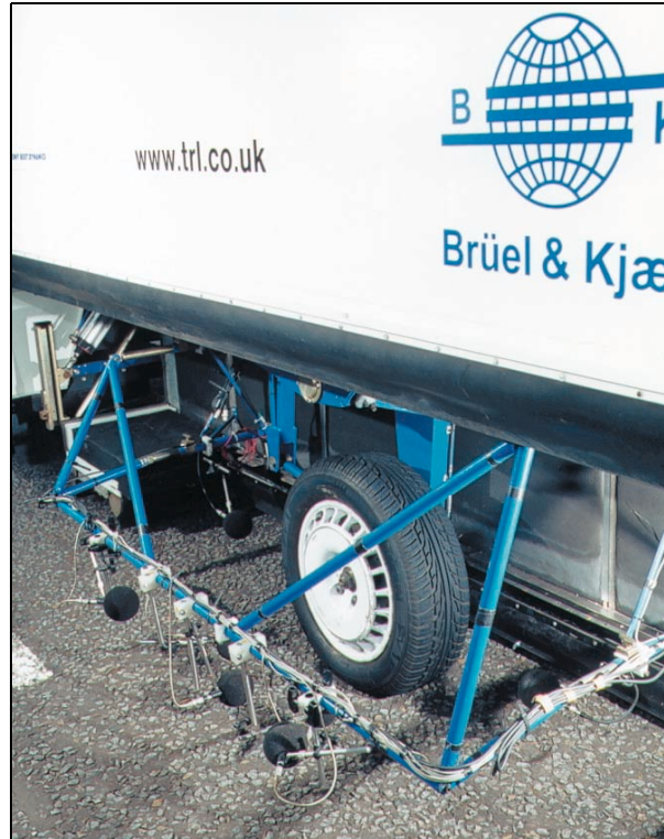
Fig. 1 The test tyre and frame carrying the microphone array
