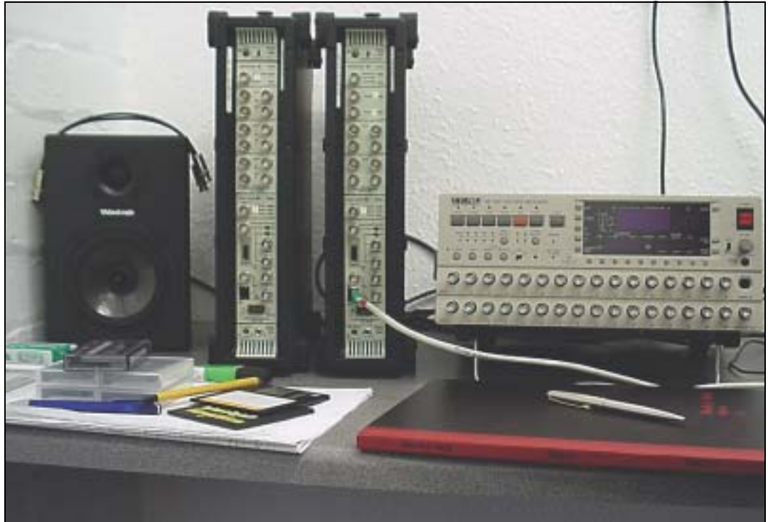
Fig. 2 Two PULSE front-ends and a 16-channel TEAC DAT data recorder
