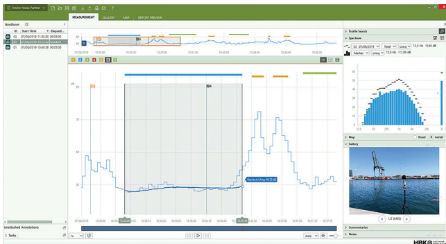
Fig. 2 Select a marker in the logging profile to view its level evolution and frequency analysis
