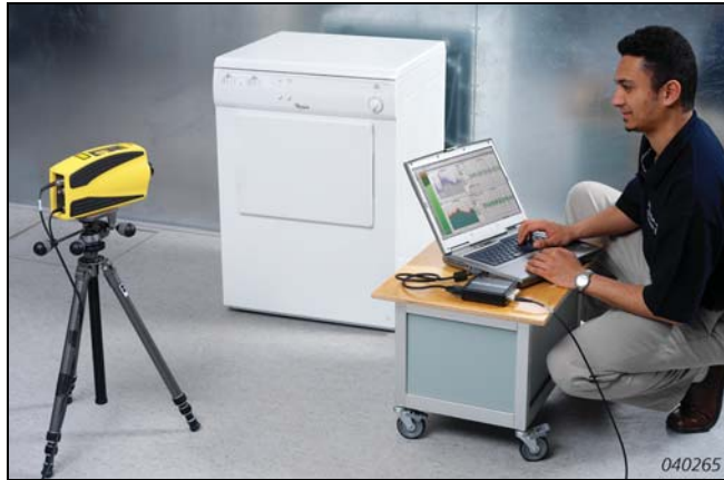
Fig. 1 Measuring on a washing machine with Type 8338
