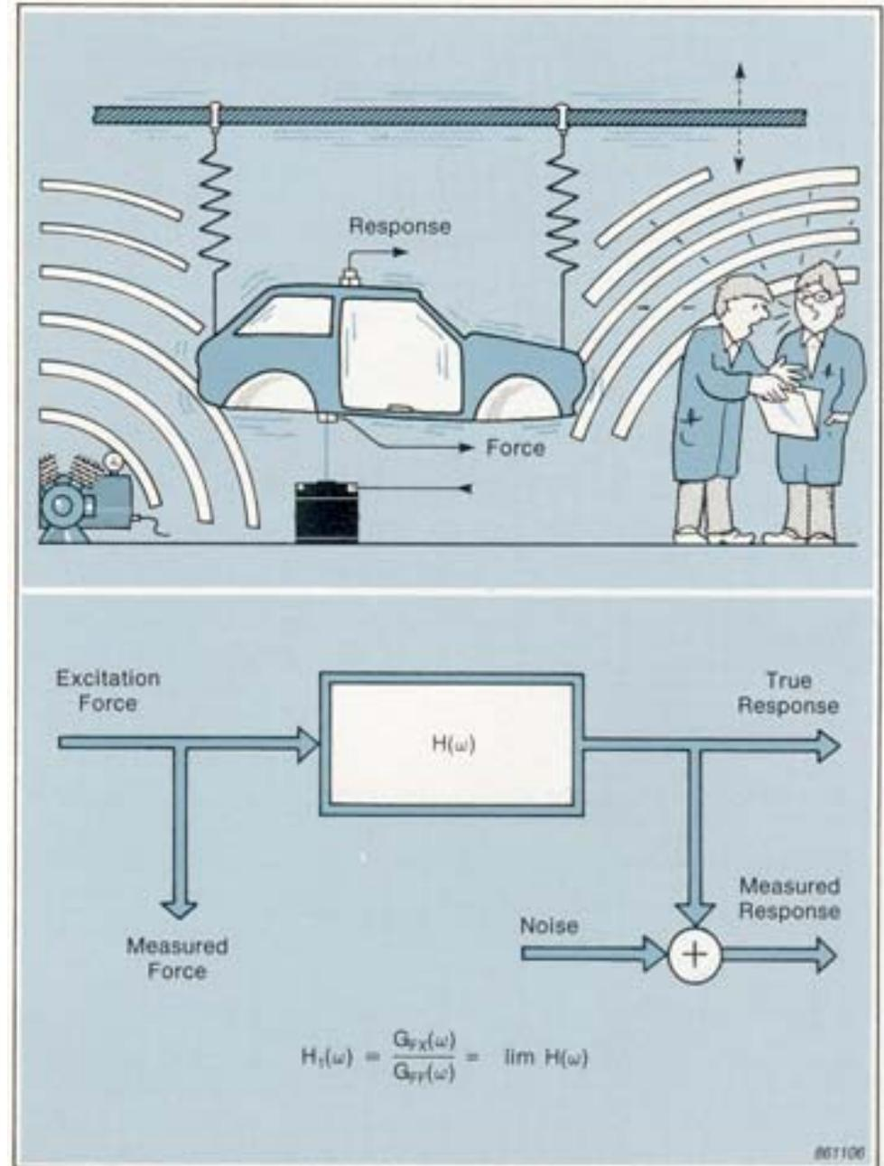
An important point about  $H_1$  is that random noise in the output is removed during the averaging process of the Cross Spectrum. As the number of averages is increased,  $H_1$  converges to the true  $H$ .
