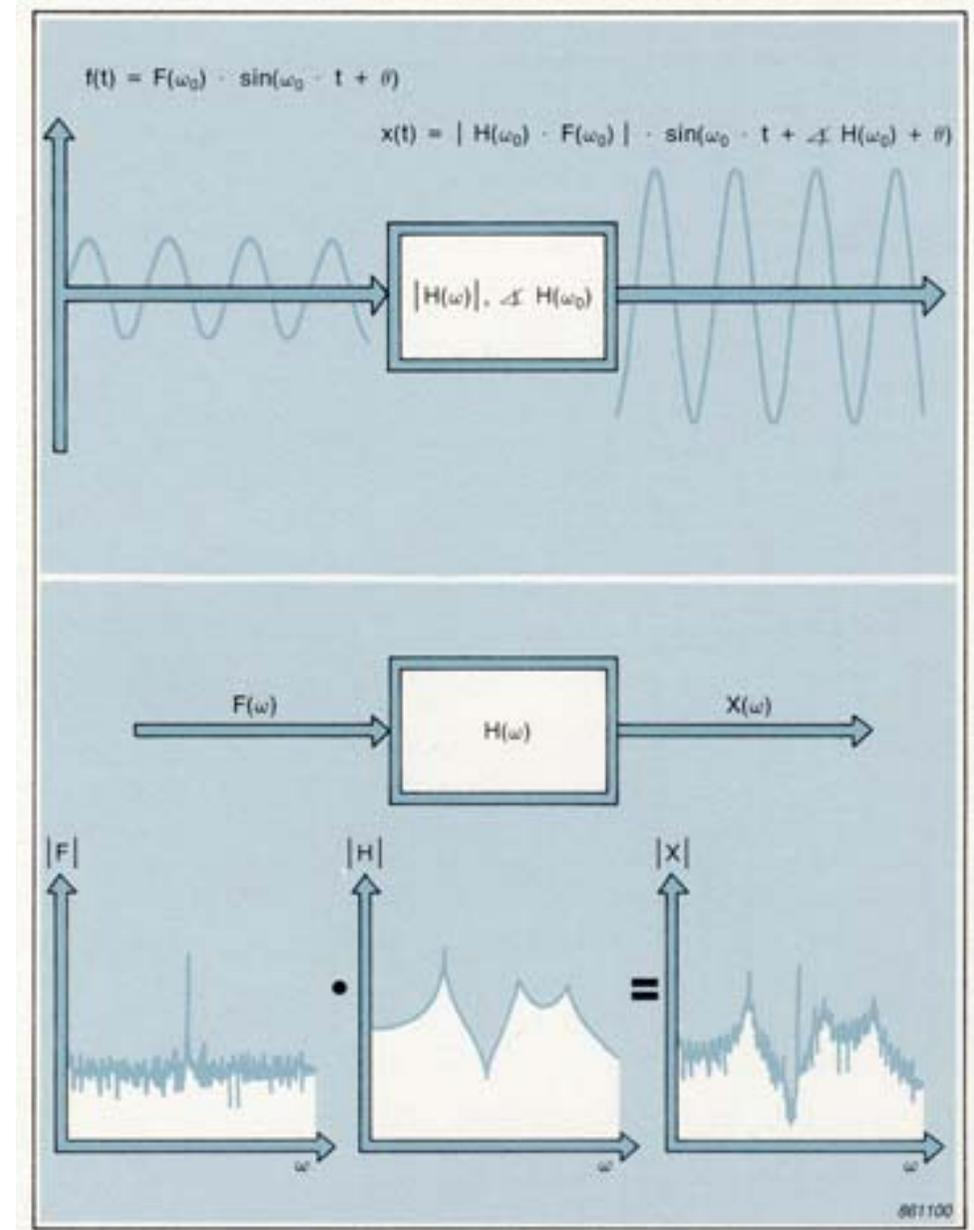
The definition of the FRF means that, in measuring a specific function, the measurements can be made sequentially at discrete frequencies or simultaneously at several frequencies. A useful technique is to use a wide frequency bandwidth for the excitation force. This gives a dramatic reduction in measurement time, as compared to sinusoidal excitation where one frequency is measured at a time.
