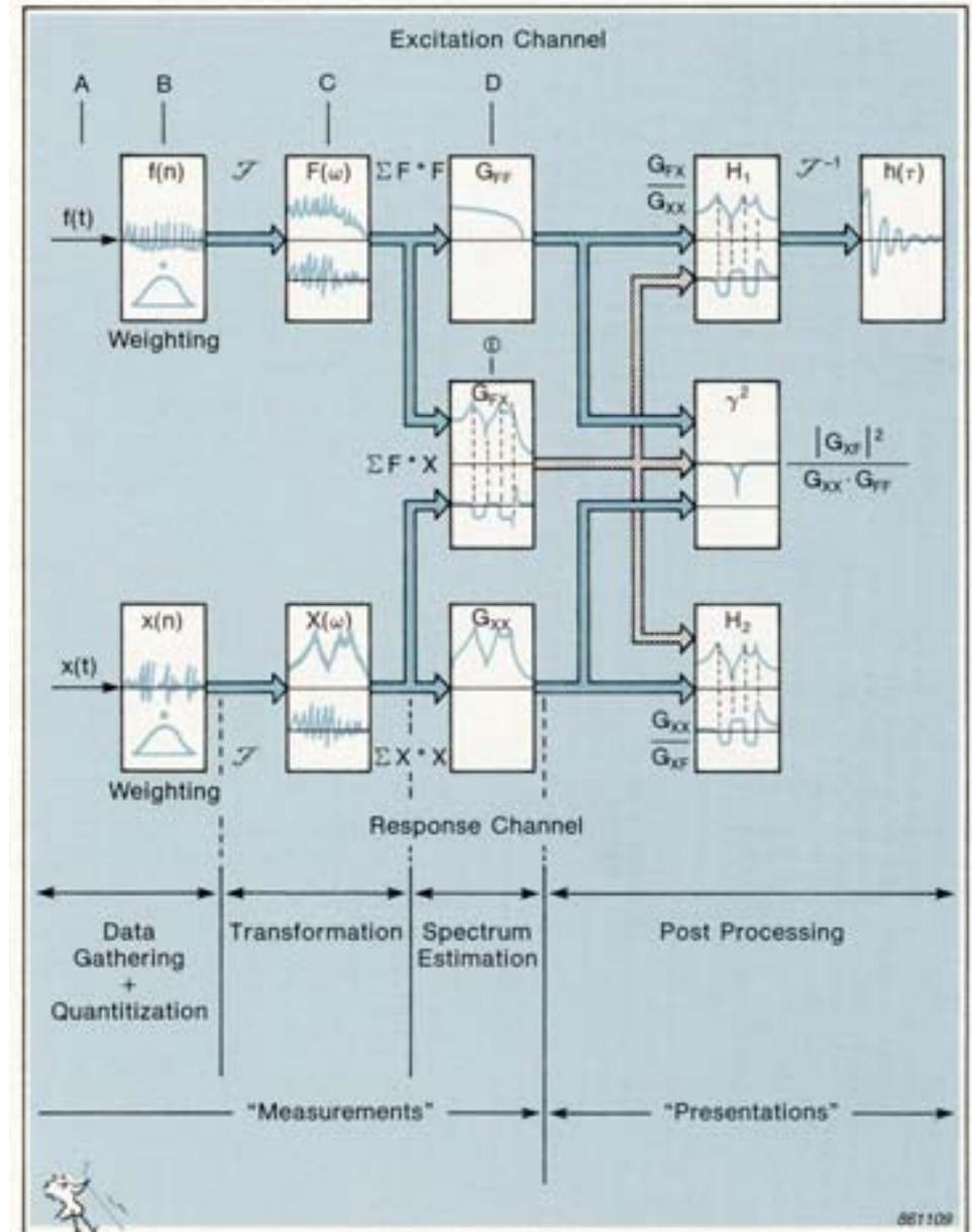
D) An Autospectrum is calculated by multiplying a spectrum by its complex conjugate (opposite phase sign), and by averaging a number of independent products.
