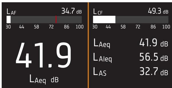
**SLM view** (left) and **List view** (right) are the main displays for single measurements. SLM view shows a bar graph and one broadband parameter. List view shows a bar graph and a list of broadband parameters.
