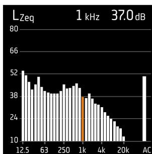
**Spectrum view** displays the frequency analysis of spectrum parameters, shown as decibel (dB) levels by Hertz (Hz).
