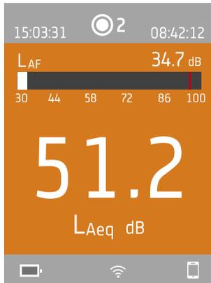
Press ▲ and ▼ briefly to scroll through measurement displays. Press ◀ and ▶ briefly to scroll through the parameters for each display.
