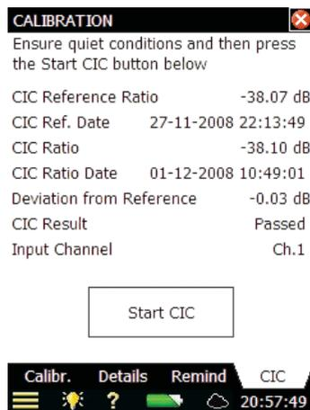
The result of the Charge Injection Calibration consists of four parameters:
