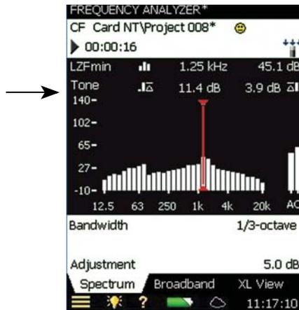
The information shown in the value panel can be changed by tapping in the field. From the tone parameters, the adjustment and the selected tone standard can be selected. See Fig. 13.7.
