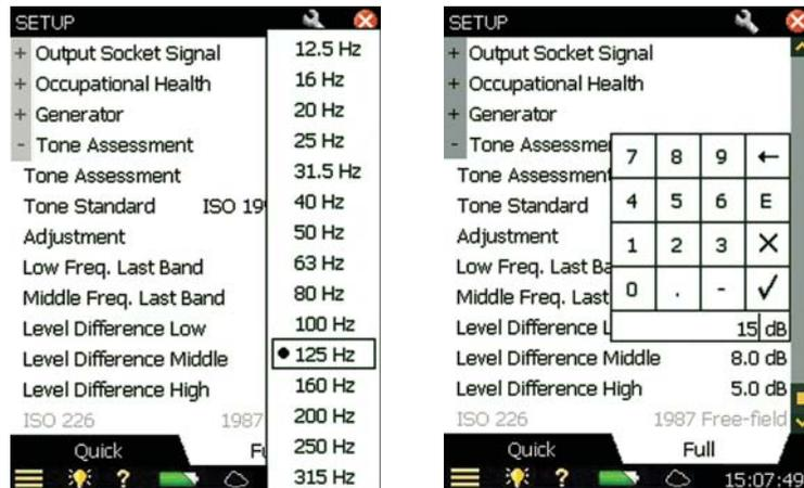
You set the division between the Low/Middle frequency range by selecting the required value for the *Last* (or highest) *Band* in the low frequency range (from 12.5 Hz to 315 Hz), and set the division between the Middle/High frequency range by selecting the required value for the *Last* (or highest) *Band* in the middle frequency range (from 160 Hz to 20 kHz).
