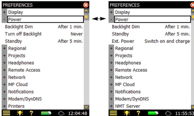
The backlight will be switched on as soon as you operate the analyzer, either by using the keyboard or the stylus on the touch-sensitive screen. The backlight brightness will be one of the six levels set by tapping at the bottom of the screen. Tap *Minimum* for minimum brightness (and power consumption), or up to *Maximum* for maximum brightness (and power consumption). Once you have chosen the level, select *Close* to save the settings.
