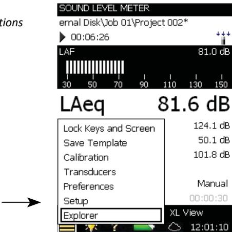
Change the broadband weighting parameters by tapping on the
