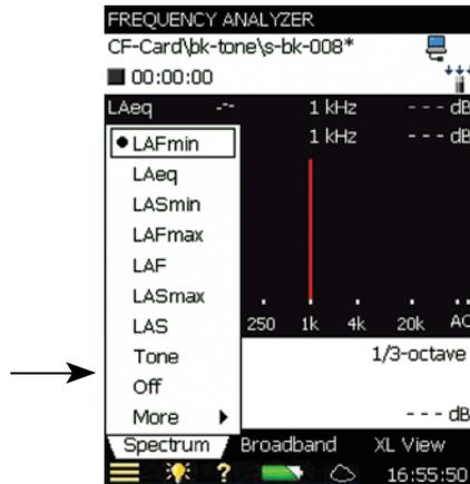
On the Results display, a blue marker is set at the top of each detected band with a tone. Differences to the left and right of the frequency band selected by the main cursor are shown (on the left and right) in the tone parameter panel above the spectrum, see Fig.13.6. The main cursor is moved using either the hard keys or the stylus.
