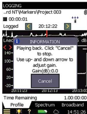
\* Playback on the analyzer is available only with G4 analyzers. If you have a G1 – 3 analyzer, you can playback recordings on a PC using Measurement Partner Suite BZ-5503. See section 12.2.5 for more information.
