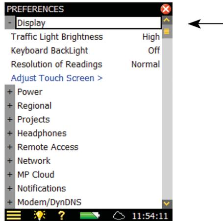
You can select the optimum choice of brightness for the traffic light (for example, *High* in bright light conditions and *Low* in dark conditions) and you can select whether to have backlight on the keyboard, or not. In very bright lighting conditions you will not be able to see the backlight, so set it to *Off* to save some power.
