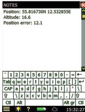
If you do not have a GPS receiver, but know the position (for example, from your smartphone), you can manually key in the position in the GPS note.
