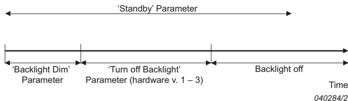
If the analyzer is left unused, not measuring and not communicating over the USB interface, it will go to standby after the time specified in the *Standby* parameter. If the analyzer is in standby mode, you must press to switch the analyzer on again.
