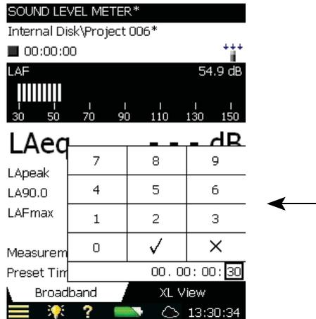
Tap on the digits or use **Up Arrow** ▲ / **Down Arrow** ▼ to increment/decrement the number. Use **Left Arrow** ← / **Right Arrow** → to select other digits if necessary. Press the **Accept** pushbutton (⊙) or tap ✓ on the number keyboard to enter the number for the parameter. Tap ✗ on the number keyboard, or outside the number keyboard to cancel the change of value.
