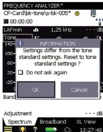
The pop-up window can be deactivated for the rest of the measurement session. To activate it again, you will have to reload the template or restart your analyzer. This automatic check is deactivated when
