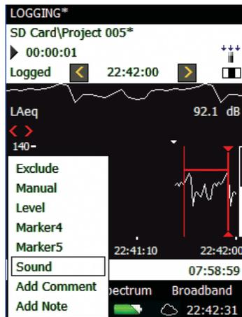
The small triangle above the profile indicates the amount of sound you have in the internal buffer – ready for storage in a wave-file. You will have sound from this triangle to the right-hand side of the profile. The triangle is updated every second.
