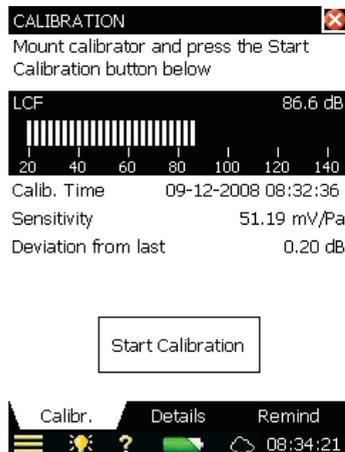
This screen contains a bar graph showing the actual sound pressure level and three placeholders for displaying information about the last calibration.
