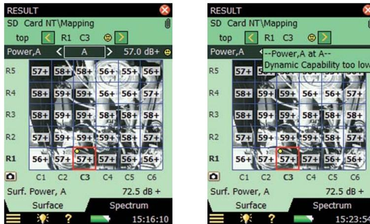
15) Tap **Spectrum** to display the spectrum at R1, C3. Note that the dynamic capability is too low for 80 Hz only in this segment. Because it does not have any effect on the Power for the surface, there is no smiley for the *Surf.Pwr,A* readout (Fig.3.40).
