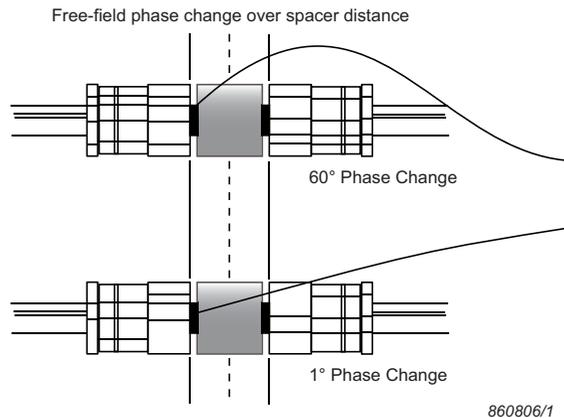
These problems can be reduced by using a longer spacer between the microphones, but as stated in section 6.12.1, this will reduce the high frequency limit.
