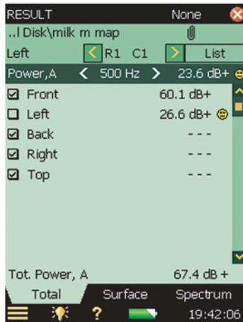
The Total display lists the surfaces defined in the project (Fig.5.55): one reading from each surface. Use the check box to include/exclude the entire surface from the calculation of the total power.
