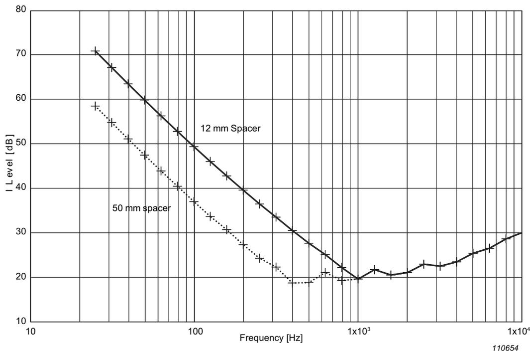
The curves in Fig. 6.73 consist of two parts: The decreasing part at low frequencies and the slightly increasing part at high frequencies. The first part is the sound intensity part. It is limited by the spread in the sound intensity measurement. The second part is the sound pressure part. It is limited by the bias error in the sound pressure measurement. Only the sound intensity part can be lowered if the averaging time is increased.
