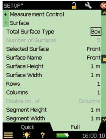
According to ANSI S12.12, two measurement surfaces must be defined around the source under test, one divided into  $N/2$  segments, the other divided into  $N$  segments ( $N \geq 8$ ).
