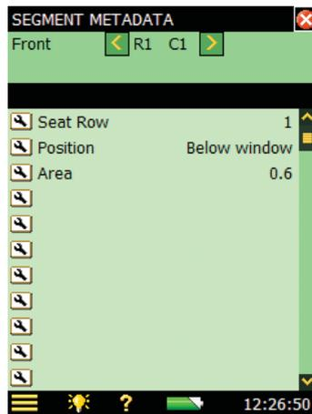
At the top of the display (Fig.4.47) are the surface selector and segment selection arrows for selecting other surfaces and segments.
