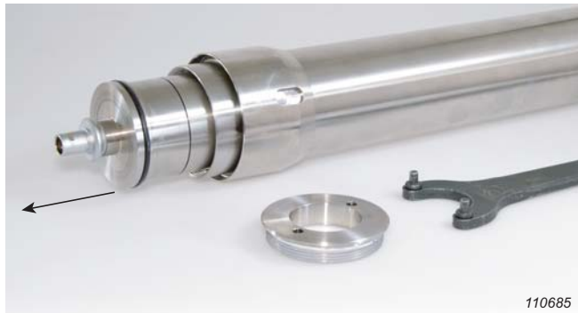
Fig.D.6 Slide the electronics assembly out of the microphone housing
