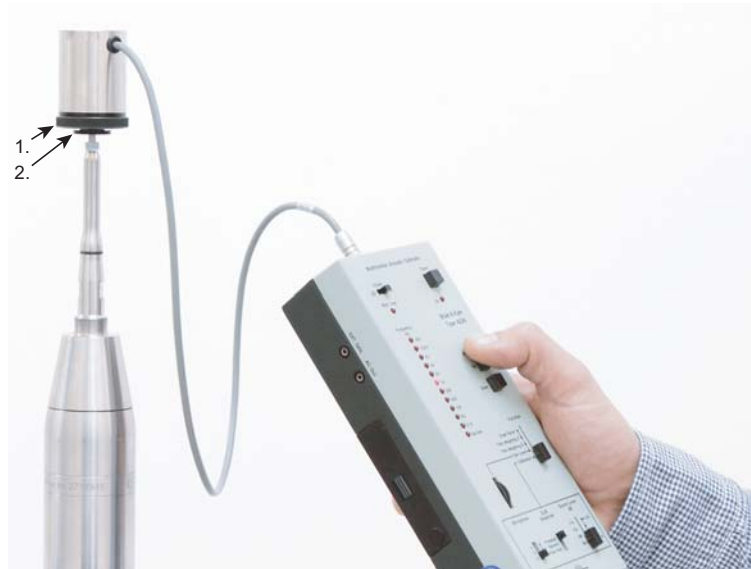
Fig. D.4 Weatherproof Microphone Unit Type 4184-A and Calibrator Type 4226 with 1. Acoustic Coupler UA-1231 and 2. Calibration Adaptor DB-4199
