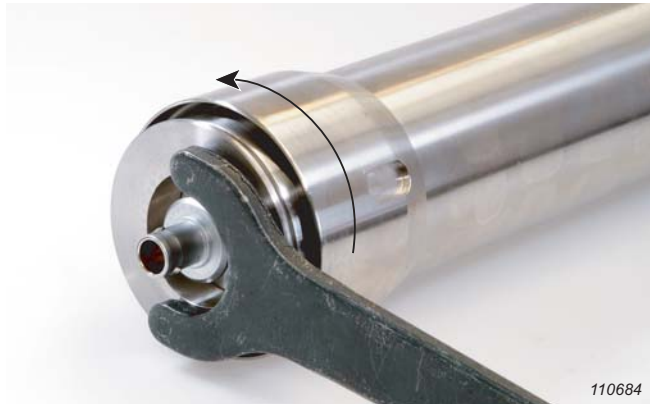
Fig.D.5 Base of Type 4184-A and pin wrench: Unscrew counter- clockwise
