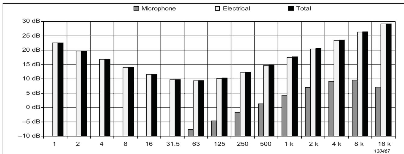
**Fig. 4.25a** Typical self-generated noise, 1/1-octave band, High Range, without UC-0211
