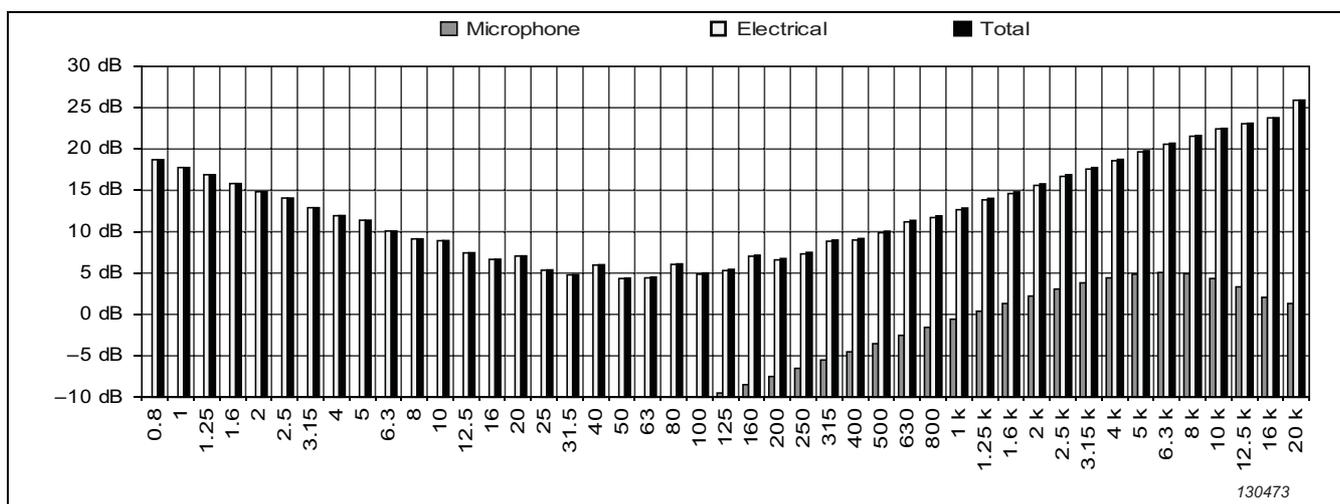
**Fig. 4.28a** Typical self-generated noise, 1/3-octave band, High Range, without UC-0211
