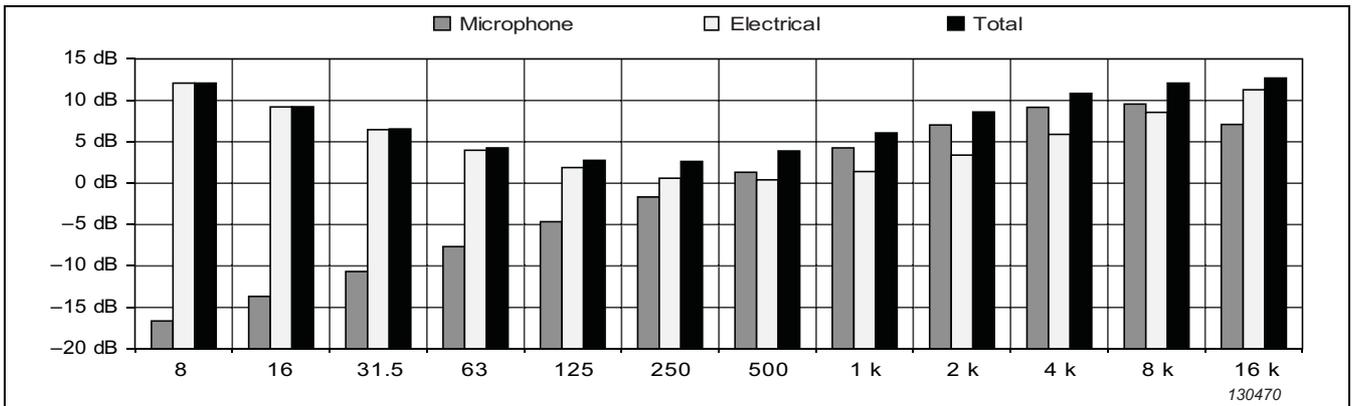
**Fig. 4.26b** Typical self-generated noise, 1/1-octave band, Low Range, with UC-0211
