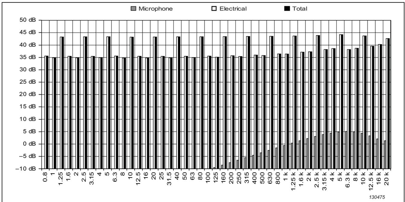
**Fig. 4.29a** Typical self-generated noise, 1/3-octave band, Low Range, without UC-0211
