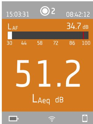
In the middle is the measurement display. There are views for broadband parameters (SLM view and List view), spectrum parameters (Spectrum view), reverberation time measurements (Reverberation time view) and a view for information about your data (About data view).
