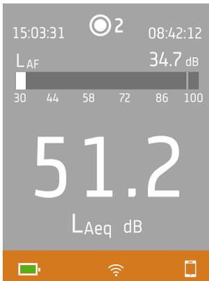
The bottom region provides information about the system: battery, network, and connectivity status.
