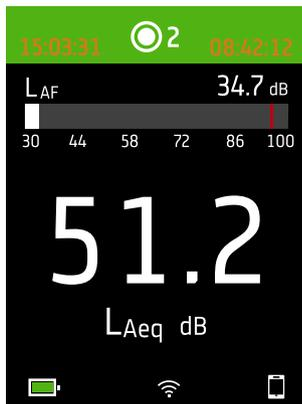
During a measurement, the instrument displays the start time (to the left) and the elapsed time (to the right).
