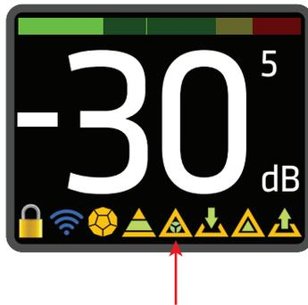
If the fan is forced off while, based on the loudspeaker power stage temperature, the fan control would have turned it on, the fan icon will turn red. The colours of the fan icon give a basic indication of the fan control settings.
