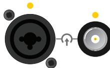
Inputs can be balanced or unbalanced and equipped with an input amplifier and/or power supply. Compared to unbalanced signal connections, balanced connections are better able to cancel out AC ground loop hum or picked-up radiated interference that might emerge with low-level signals. On the other hand, unbalanced connections are usually simpler.
