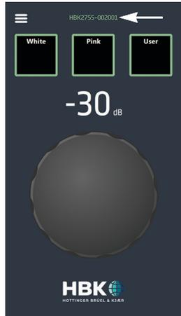
To start signal playback, click a generator button with the cursor. The button frames will turn red momentarily while the command is being sent to the amplifier. Once the signal playback is started, the button for the active signal turns green.
