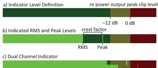
In situations where high-level energy spectra are more important than low distortion, it may be preferred to have the clipping border crossed and let a fraction of the signal peaks clip at the power output. This is, for instance, true for external noise signals that are normally set at high levels in sound insulation measurements.
