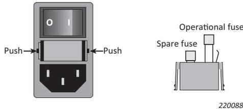
**Please note:** After replacing the operational fuse, do not forget to replace the spare fuse too. Littelfuse® T 5 AH 250 V 215 series fuses (part number 215005.MXP) are recommended.
