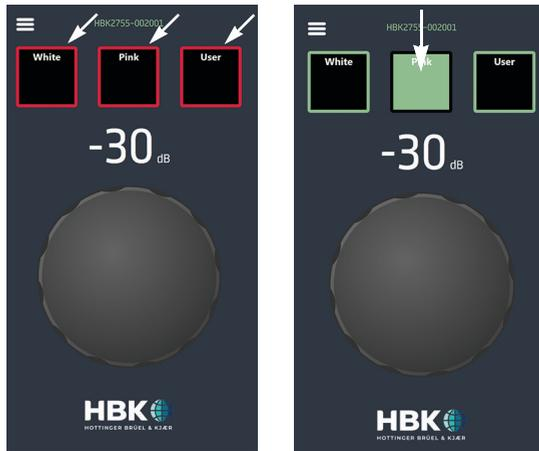
To change the attenuation, turn the attenuation knob by swiping the cursor from the bottom left to the top right and back again (click+drag on a laptop). While the changed attenuation value is being sent to the amplifier, the displayed value shortly turns red.
