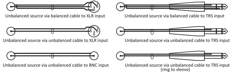
**Please note:** An unused pin of a balanced input may also be connected to ground, as shown with the bottom right example in the above figure, where the ring is connected to the sleeve (ground).
