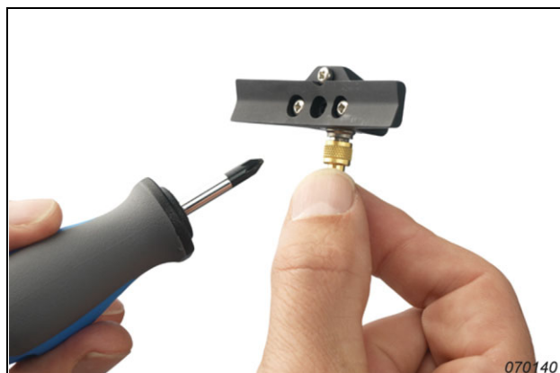
Fig. 4.5 Mounting accelerometer in adaptor
