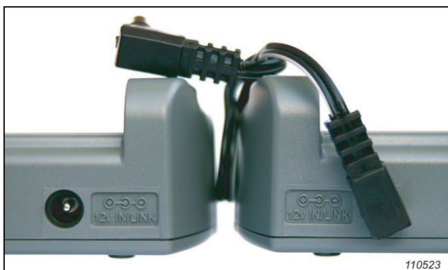
Fig. 2.3 Linking charging stations Right: Primary Left: Secondary
