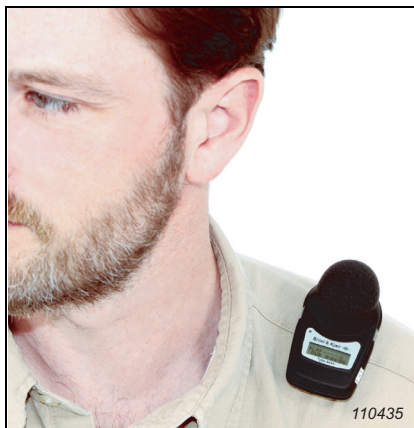
Fig. 2.4 Type 4448 mounted (with pins) on the shoulder 10 cm from the ear with the microphone approximately 4 cm above the shoulder
