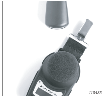
Fig. 4.5 Type 4448 and IR sensor positioned for data transfer
