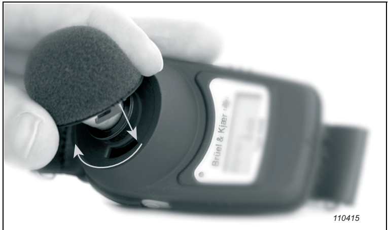
Fig. 3.3 Attaching the windshield
