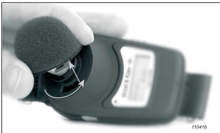
Fig. 3.1 Removing the windshield (DS-1174)
