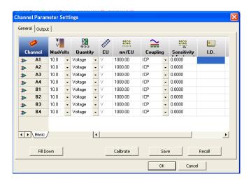
• Multi-Focus II Data display – Master unit signals designated by an "A" character. Slave unit signals designated by a "B" character
