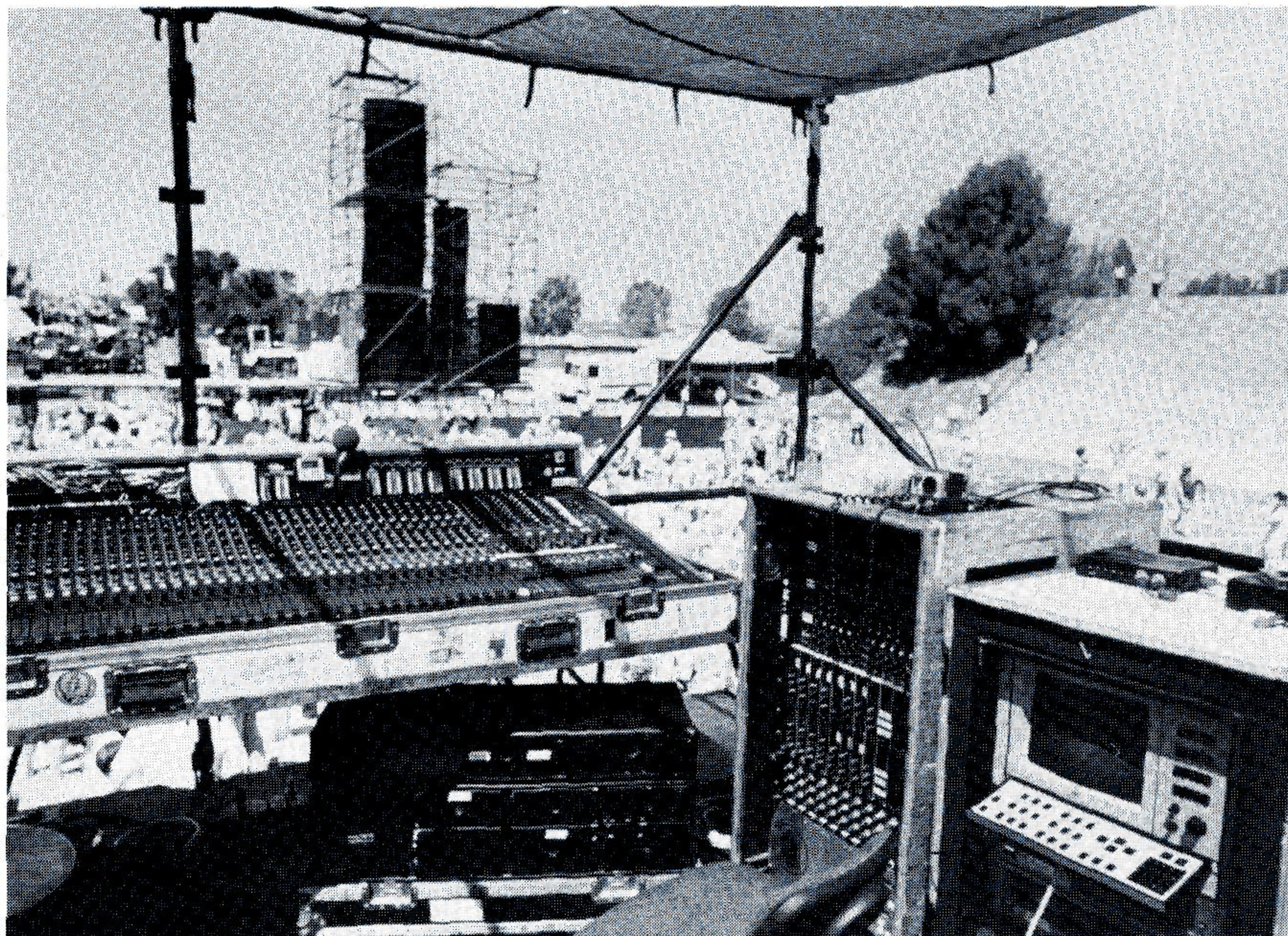
The Grateful Dead's sound system, including Dual-Channel Signal Analyzer Type 2032
