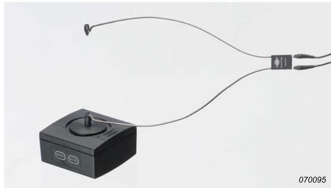
Fig. 3 Calibration of Type 4101-A using Adaptor DP-0978 and Sound Calibrator Type 4231
