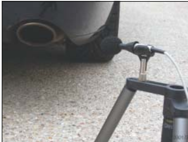
Fig. 6 External tacho setup (boot closed)
