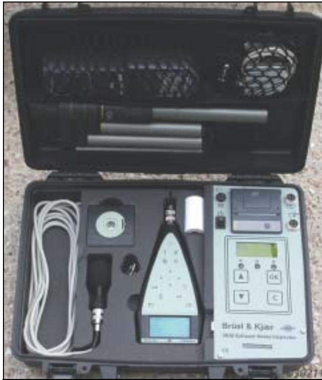
Fig. 8 Complete suitcase including SLM, calibrator and optional tachometer
