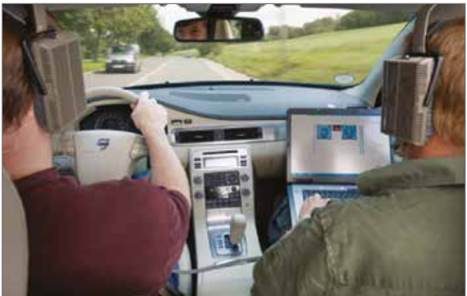
The DTS On-road simulator is used for back-to-back evaluations of benchmarked vehicles or proposed targets, while driving a real 'mule' vehicle
