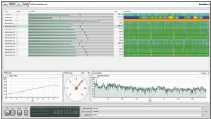
PULSE Time data recorder with coloured level history and channel monitor viewing time or frequency content. Tachometer and RPM profile readout as well as RPM triggers are essential recording tools used during a run-up/coast-down
