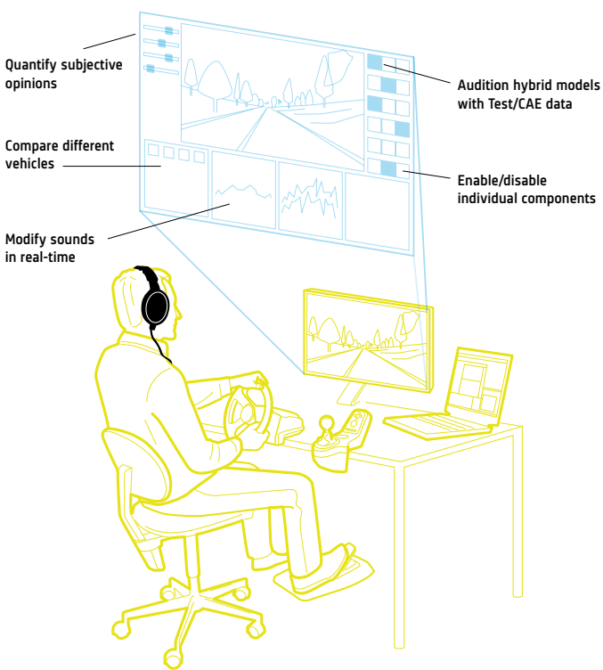
The NVH desktop simulator allows sound from vehicles, components, target levels and CAE data to be accurately evaluated in an interactive, realistic environment
