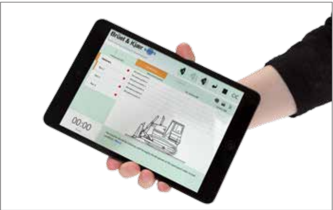
Use of tablet for remote control of sound power for earth-moving machinery application
