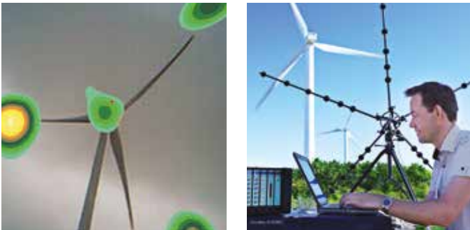
Result of sound intensity mapping from a beamforming measurement
