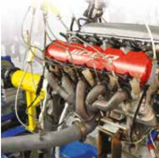
Dodge Viper 8.3L V10 engine fitted with transducers for crank angle analysis
