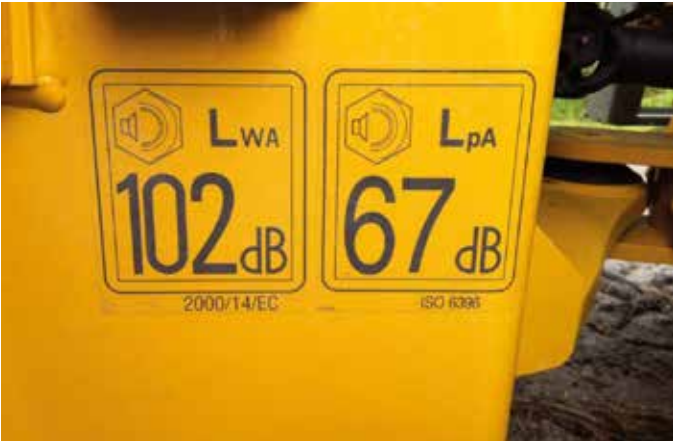
Sound power and sound pressure level values used for labelling on a back hoe loader
