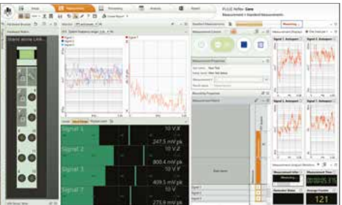
4-channel real-time FFT and Level monitoring with a single microphone and triaxial accelerometer. This measurement includes a recording in addition to the real-time measurement. This recording can be automatically post-processed through PULSE Reflex Core for additional types of analysis
