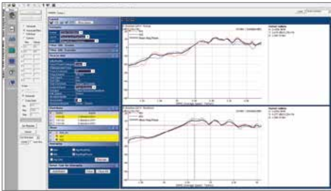
Validator provides targeted automatic retrieval of test results for averaging, reporting and comparison to other relevant measurements or target data
