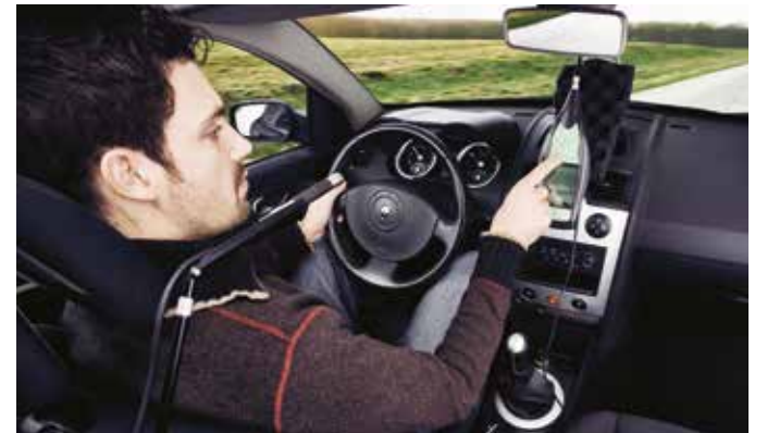
Fast and easy in-vehicle measurement of sound at the driver's right ear reference location
