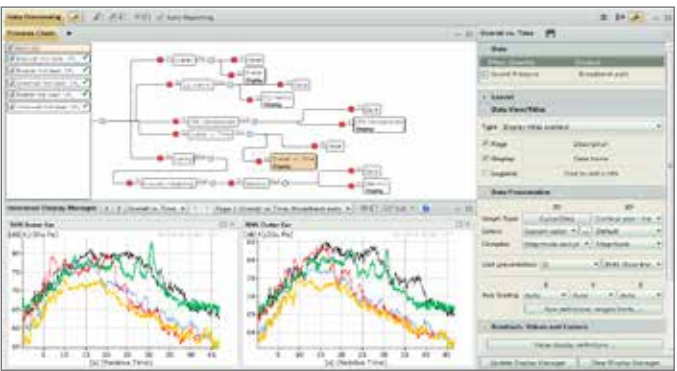
Batch post processing of multiple recordings through a user defined process chain consisting of Overall, CPB and sound quality analysis
