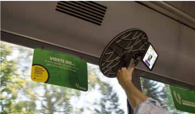
Reflex Acoustic Camera screen shot when used for troubleshooting on a hybrid motor
