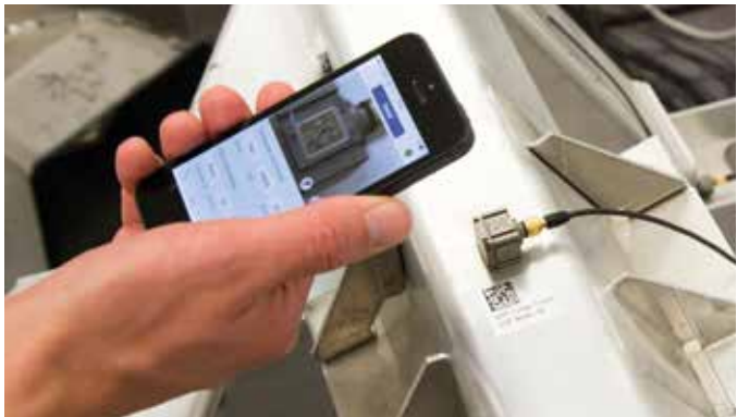
Scanning the data matrix code on the transducer (transducer information and orientation) and the label next to the transducer (transducer position and node ID) using the Transducer Smart Setup app ensures fast and correct DOF information for the measurement
