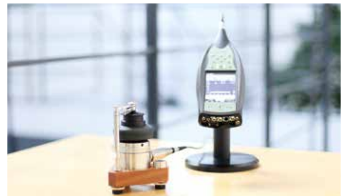
Calibration of a TDH-39 headphone with Artificial Ear Type 4152
