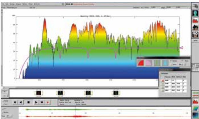
Interactive filtering, as shown here in BZ-6047, is an integral part of basic sound quality engineering
