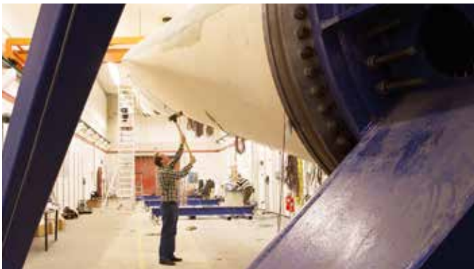
Operational modal analysis on a wind turbine blade using hammer excitation randomly in space and time. Only accelerometer responses are measured
