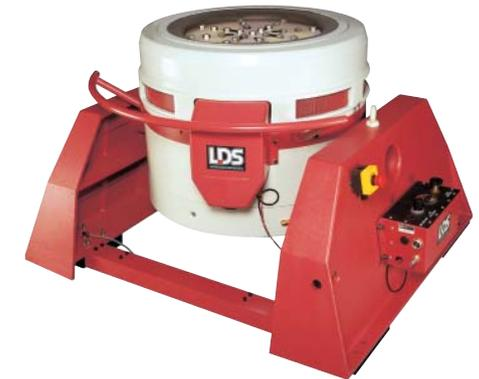
Systems are available in various forms to meet a customers exact requirements - mounted in a trunnion (standard item), or combined with a horizontal oil-film slip table, (combo base).
