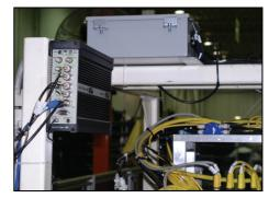
Accelerometers Type 4514-B located near each motor and in the middle of each side rail. These measure the vibration from the DC motors. In addition to the vibration measurement, a current probe clamp is also installed over the power lead to the sunroof, and the signal used to determine the RPM of the motor. The test takes about one minute. On average, the throughput is one complete sunroof system every three minutes on each production line.
