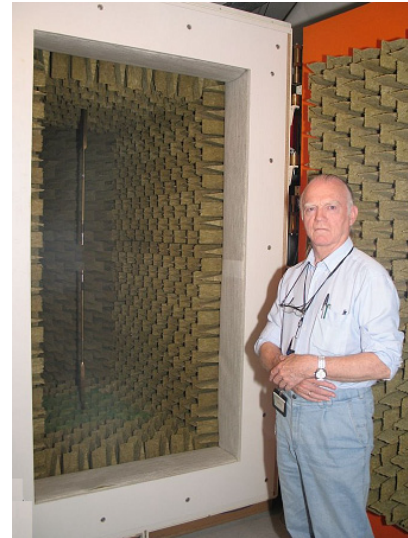
Figure 8: The DPLA-DFM free-field calibration room. The microphone mounting bars are automatically moved between pre-selected microphone positions (In front: Knud Rasmussen)
