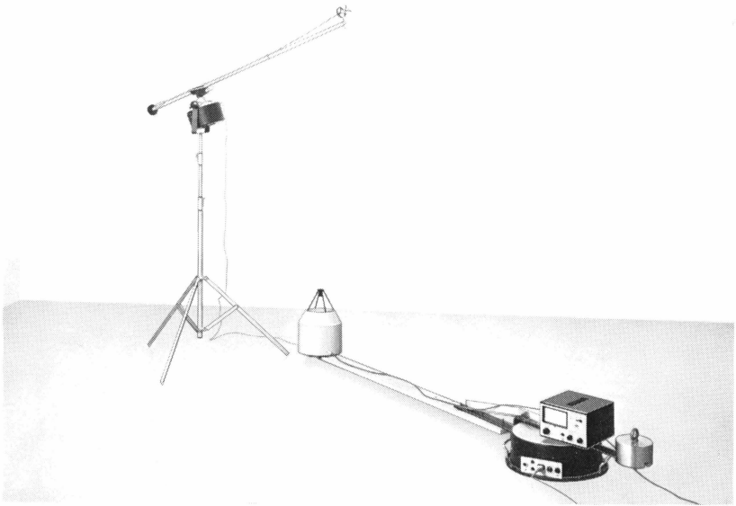
Fig.6. Measuring set-up for rotating sound source and microphone
