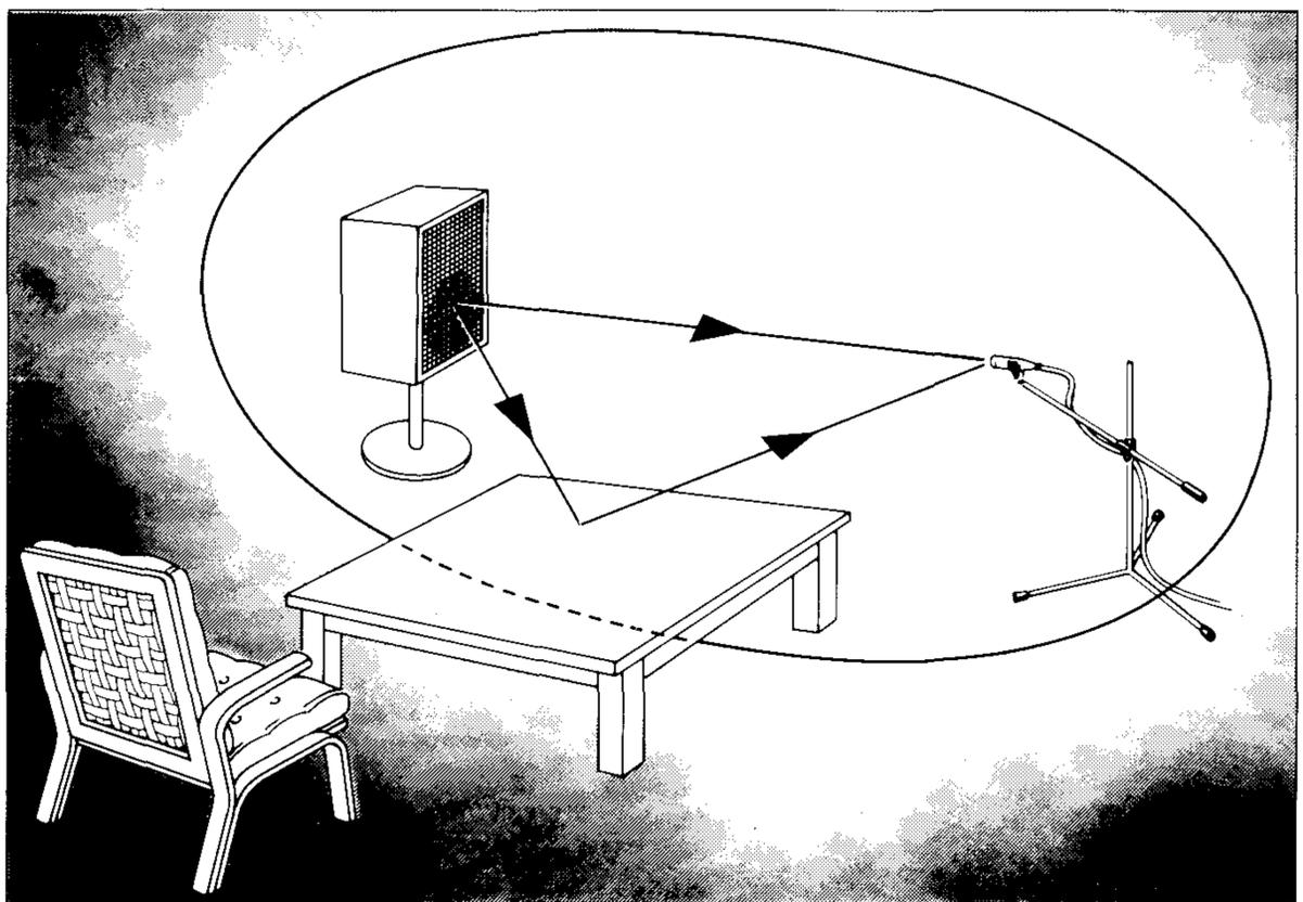
Fig.4. When the measurement technique allows the use of time gating — windowing — it is possible to isolate the direct sound from the reflections which are always present in a normal environment. Only objects which are located within an ellipsoid, the size of which depends on the length of the time window, interfere with the measurement
