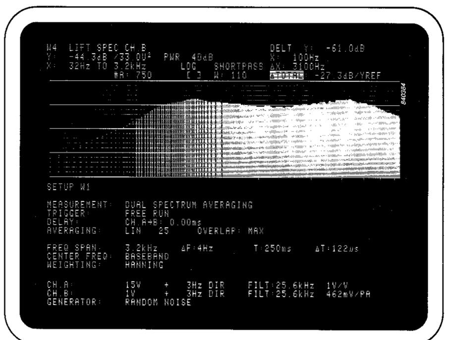
Fig. 21. Sound power output for 1 W electrical input in the frequency range 100 Hz to 3,2 kHz. The sound power is measured by averaging the sound pressure at 30 positions on a sphere ( $4\pi$  steradians) around the loudspeaker in an anechoic room. The resulting power spectrum has been "liftered" (= smoothed) for easy comparison with Figs. 16 and 17. The " $\Delta$  TOTAL" field indicates an acoustical output of  $-27.3$  dB relative to 1 W in the chosen frequency band
