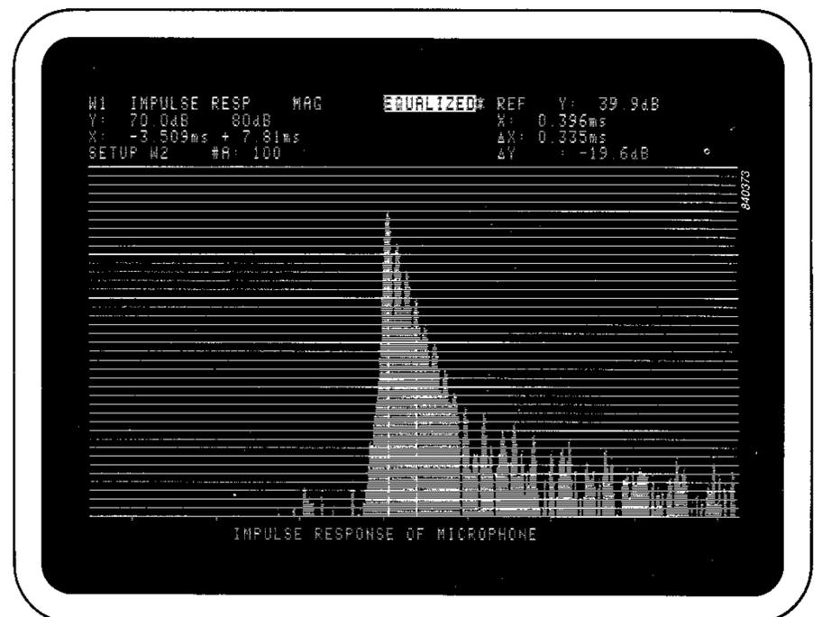
Fig. 14. Since the impulse response is obtained from the calculated frequency response rather than directly from the input data, it is also possible to extract the impulse response of a microphone from the combined response of loudspeaker and microphone. The logarithmic presentation provides direct visualization of the decay rate for the multiple reflection
