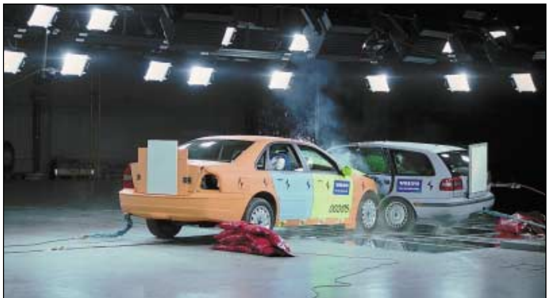
Fig. 3 At the moment of impact, digital cameras record the crash at up to 1000 frames a second. Accelerometers measure the g forces on the cars and the dummies
