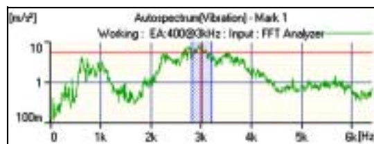
Fig. 7 Baseband FFT spectrum of bearing in lathe
