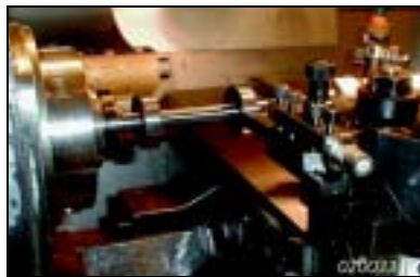
Fig. 6 Bearing mounted in lathe
