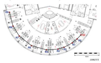
The loudspeaker source is positioned at one of the workstations (S2) and a sound level meter (SLM) is moved in turn to each measurement position (R1 – R9). DIRAC, running on a laptop, switches on the speaker test signal and instantly calculates the speech intelligibility indices from the sound level meter microphone signal. Multiple (wireless) sound level meters can significantly speed up the measurement process.
