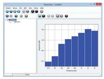
Fig. 22 Parameter graph showing  $D_{50}$  average and standard deviation over four receiver positions
