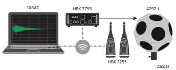
If the PC is far from the source or the microphones, a wireless setup becomes useful. Fig. 4 shows a wireless setup where the PC, sound device (HBK 2755) and one or more sound level meters communicate via Wi-Fi<sup>®</sup>.
