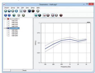
Fig. 23 Parameter graph showing  $D_{50}$  average over four receiver positions, for two different source positions
