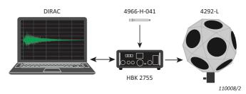
Fig. 2 illustrates the typical use of DIRAC to measure reverberation time and speech intelligibility in an open-plan office. The system components are shown in Fig. 3 and include HBK 2755 Smart Power Amplifier which can be used as a sound device (see The Sound Device on page 4).
