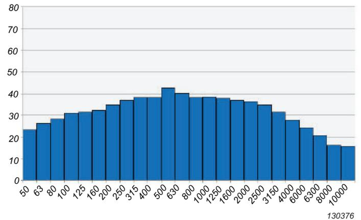
All levels are background noise corrected.  $L_{WA}$  is also corrected by  $-6$  dB to account for the approximate pressure doubling that occurs for the sound level measurements on a ground board plate, while  $L_{Aeq,c}$  is not.
