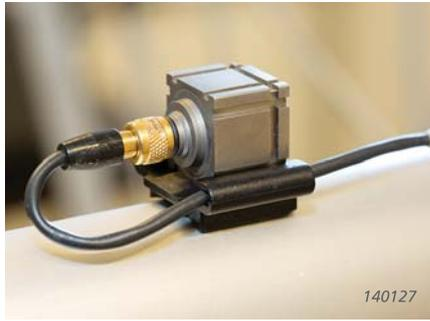
To make mounting as flexible as possible, the accelerometer housing has slots to be used in combination with a selection of mounting clips. The clips are attached to the test object with glue or double-sided, adhesive tape. This design allows the accelerometer to be easily fitted to and removed from a number of different objects, for example, during calibration. Fig. 2 shows the slots, connector orientation and dimensions of Type 4529.
