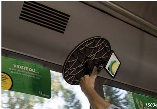
Fig. 4 Left: Hand-held Array WA-1764-W-001 with reflective plate for use in beamforming measurements Right: Without reflective plate for use in acoustic holography measurements
