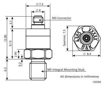
Type 4385-C is a piezoelectric accelerometer with a centre-mounted compression design. It features an M3 output connector (top) and an integral M5 mounting stud.
