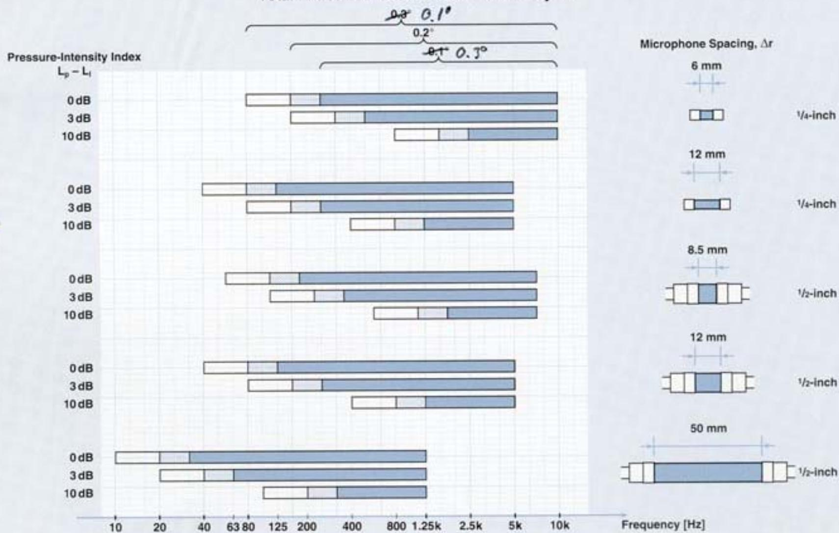
Frequency Ranges for a measurement accuracy of 1dB as a function of Pressure-Intensity Index, Microphone Spacing and Phase Mismatch
