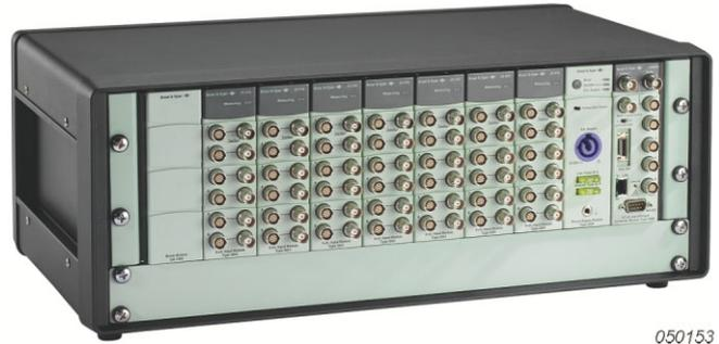
Type 3560-E is a rack-mounted data acquisition system comprising 10 modules. One of these must be the DC Power Supply Unit Type 2826, and one must be a Controller Module. The remaining 8 modules can be freely chosen from the I/O modules (see Fig. 1)<sup>a</sup>.
