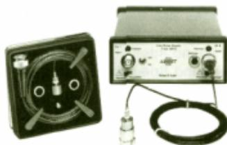
The Brüel & Kjær Line Drive Amplifier is a miniature, unity-gain signal conditioning preamplifier, which can be mounted directly onto the top face of B & K accelerometers equipped with top connectors, or adjacent to accelerometers with side connectors.
