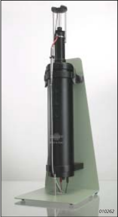
Fig. A2. Photograph of the high-pressure calibration chamber
